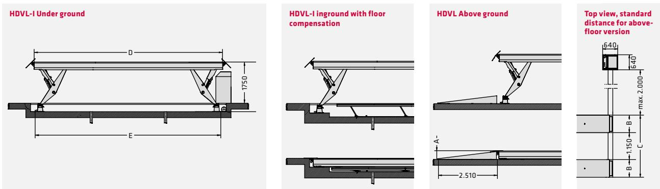
Optionally, additional long access ramps (3.300 mm) make easy driving on the guiding rails possible, even with low-floor vehicles.
