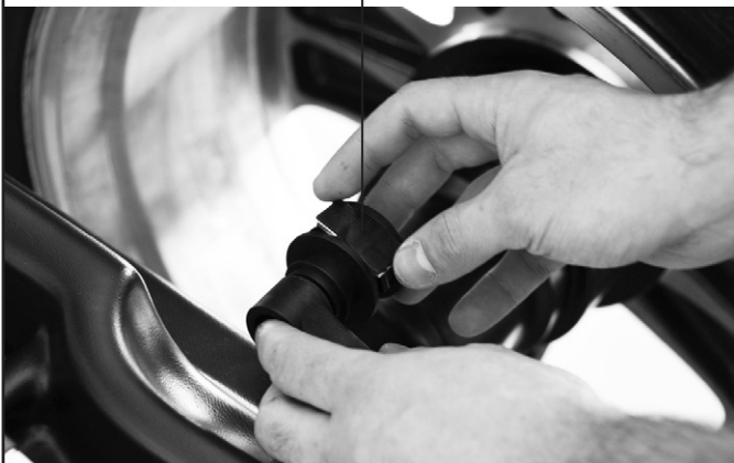
Fig. 32 Fit the adhesive weight in the pliers of the gauge rod
