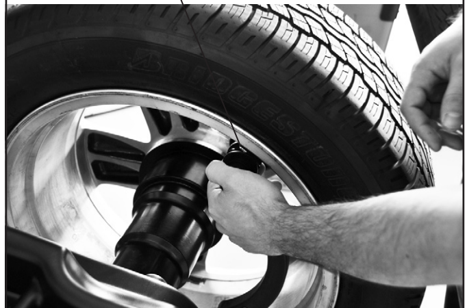
Fit weight on the position where weight pliers touches the wheel
