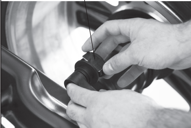
Fig. 45 Fit the adhesive weight in the pliers of the gauge rod
