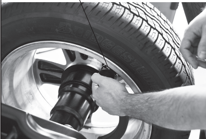
Fit weight on the position where weight pliers touches the wheel Fig. 46
