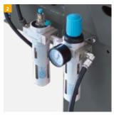
Removable pedal unit for easy maintenanceMaintenance unit with pressure regulator
