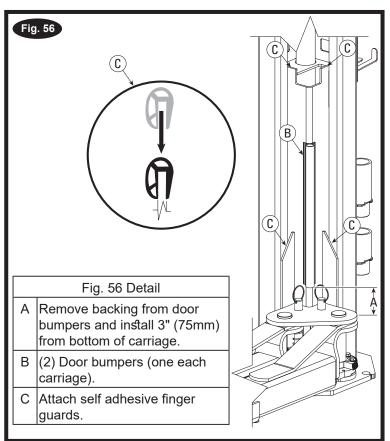
• Pinch Point Decal / Capacity Decal Location:
