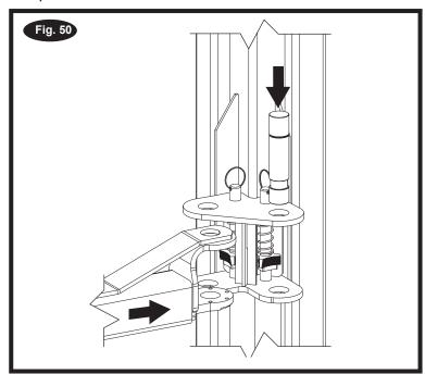
To check operation of arm restraints, raise carriage 25 cm. from full down position. Pull up on pin-ring and adjust arms to desired po sition. To engage restraint, let pin-ring down allowing gear teeth to mesh together. It may be necessary to rotate arm slightly to engage gear teeth.
