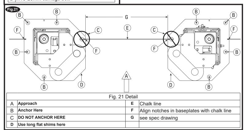
3. Concrete and Anchoring: Concrete shall have a compression strength of at least C20/25 and a minimum thickness of 200mm. Drill (8) holes with required diamter in concrete floor, using holes in column base plate as a guide. See Fig. 22. Detail information, please contact customer service.
